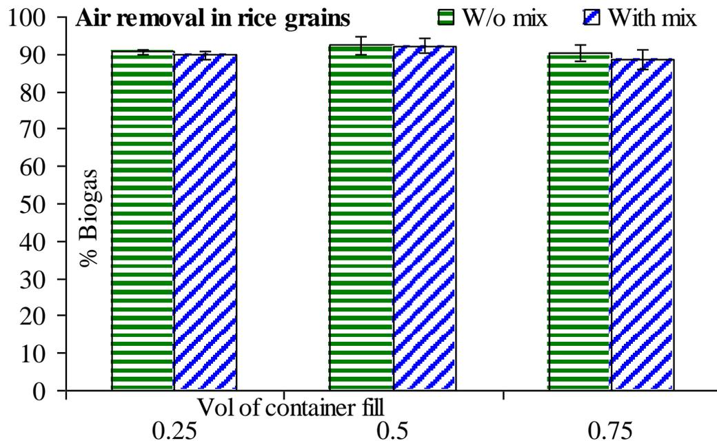
Figure 3a: Impact of the rice grain fill volume 25 % (0.25), 50 % (0.5) and 75 % (0.75) on the extent of air flushed out of the test containers for rice grains.
