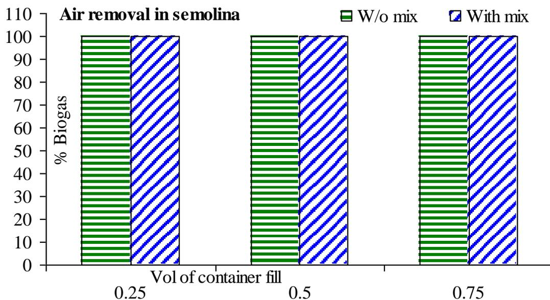
Figure 3b: Impact of the Semolina fill volume of 25 % (0.25), 50 % (0.5) and 75 % (0.75) on the extent of air flushed out of the test containers for Semolina.
