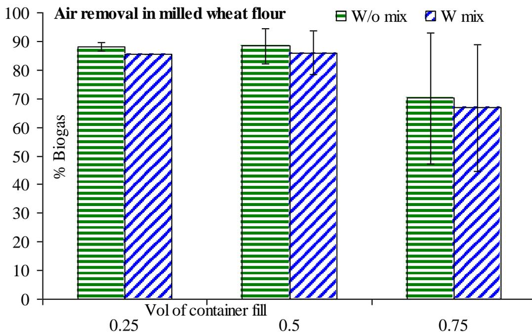
Figure 3c: Impact of the milled wheat flour fill volume of 25 % (0.25), 50 % (0.5) and 75 % (0.75) on the extent of air flushed out of the test containers for milled wheat flour.
