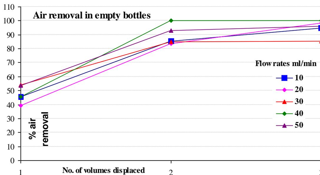
Figure 2: The extent of air displacement achieved at different flow rates and gas displacement volumes achieved.
