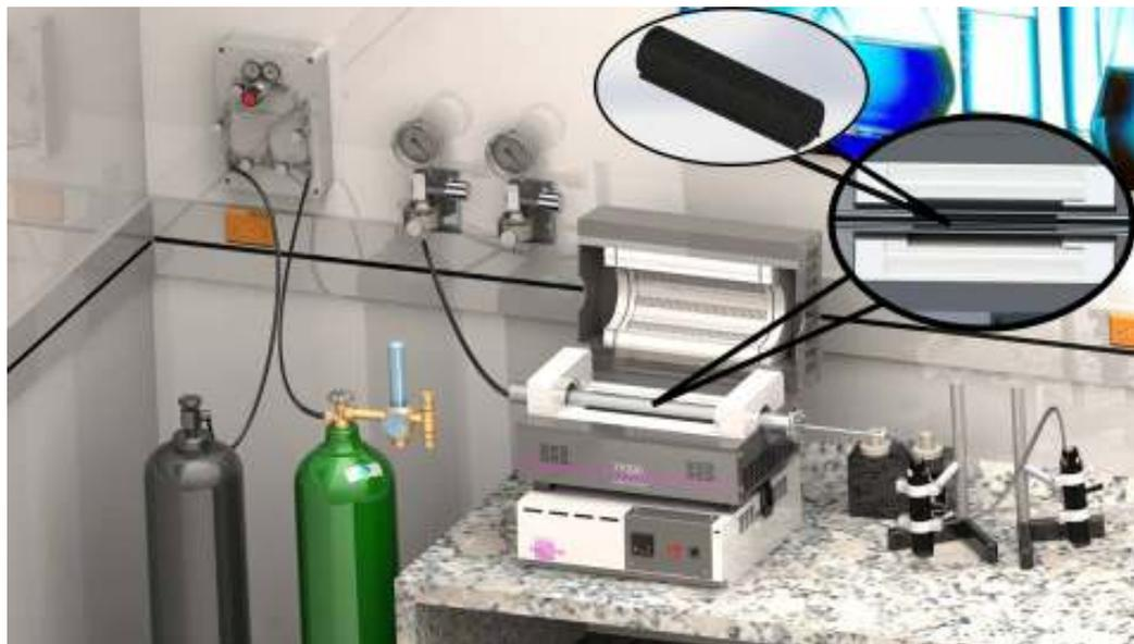
Figure (1): Set up for carbonisation and the activation of corncobs: Parts a) Nitrogen gas and Oxygen gas, b) Feed valves, c) Gas Flowmeter, d) Reactor, e) Sample holder, f) Furnace, g) Gas cleaning filter system, h) Gases to vent.
