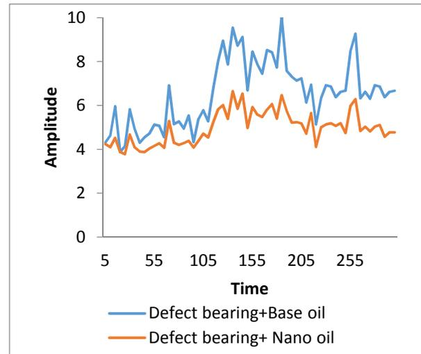
Figure (3b): Amplitude of vibration for defected bearing
