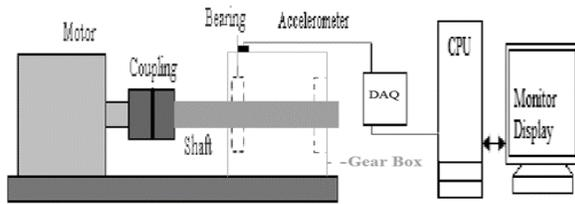
Figure (2) Test rig setup
