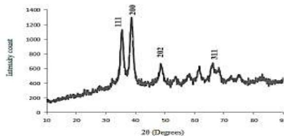
Figure (1a): XRD pattern of CuO nanoparticles
