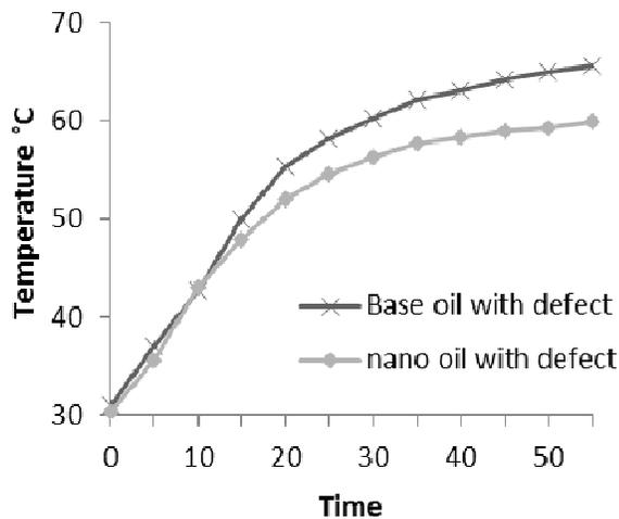
Figure (4b): Defect Bearing Temperature as function of time
