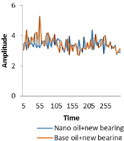
Figure (3a): Amplitude of vibration for new bearing
