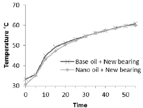
Figure (4a): New Bearing Temperature as function of time
