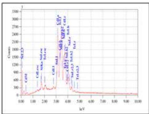
Figure (8) : EDS of CdTe thin film on FTO by electrochemical synthesis. The atomic % of Cd and Tee were shown in EDS as Cd = 33.93 % while Te = 25.23 % which deposited on copper substrate
