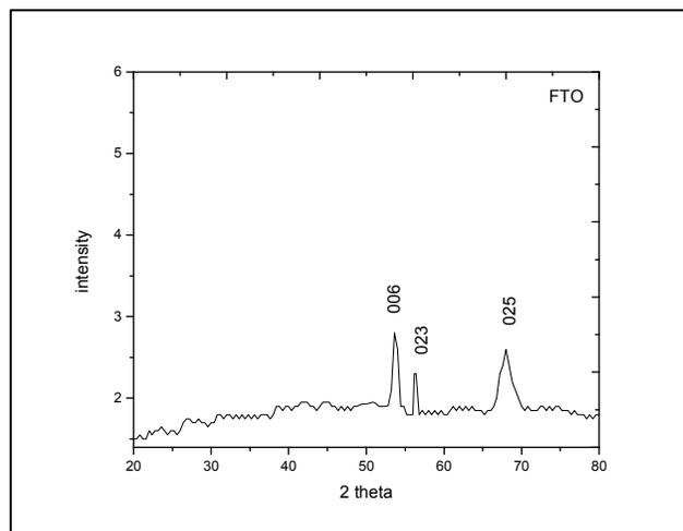
Figure (6) : XRD pattern of CdTe on FTO by electrochemical synthesis for 10 min compare with standard JCPDS data card No. 80-0090.
