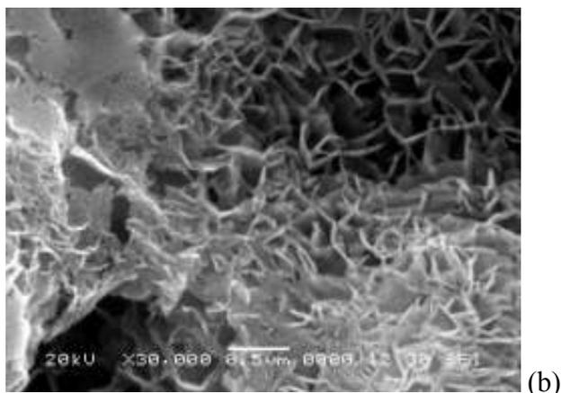
Figure (5) : SEM structure of CdTe thin film as-deposited on conducting surface (Zn) via electrochemical synthesis by simple two electrode method at pH 2.8 for 10 min (a) at low magnification X10000 (b) higher magnification X30000.
