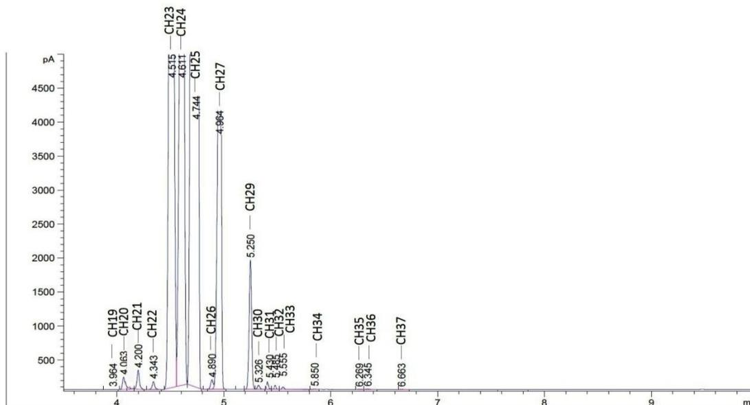
Figure (3): Gas chromatogram of used engine oil treated with *Brevibacillus* sp. AVN13 for 20 days.
