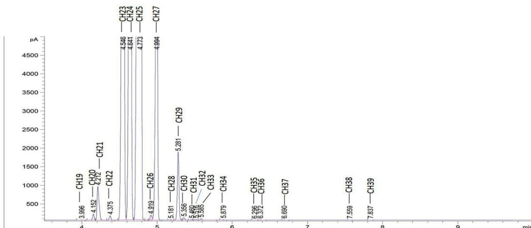
Figure (2): Gas chromatogram of used engine oil treated with heat killed *Brevibacillus* sp. AVN13 cells.
