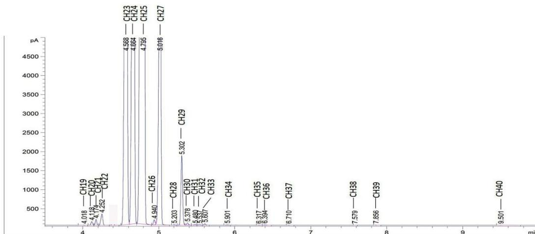
Figure (1): Gas chromatogram of untreated used engine oil (Sterile Control).
