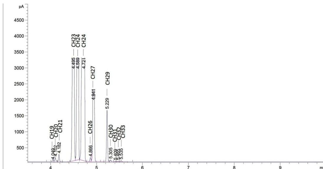
Figure (4): Gas chromatogram of used engine oil treated with *Brevibacillus* sp. AVN13 and supplemented with purified biosurfactant (80 mg/L).
