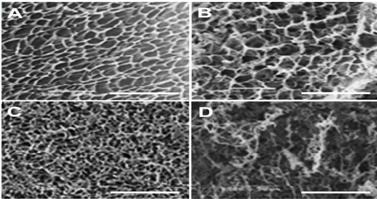
Figure (2): SEM images of (A) Polymeric network with acrylamide monomer (AM) 0.0 %, (B) Polymeric network with AM 5.0 %, (C) Polymeric network with AM 10.0 %; and (C) Polymeric network with AM 12.5 %. Scale bar represent 500 nm.
