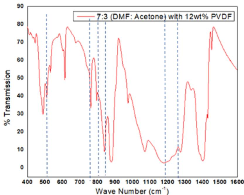
Figure (3): FTIR spectra from the sample containing 12wt% PVDF and 70% DMF (7:3)
