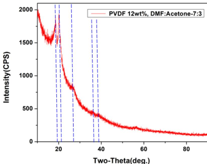
Figure (2). XRD pattern from sample containing 12wt% PVDF and 70% DMF (7:3)
