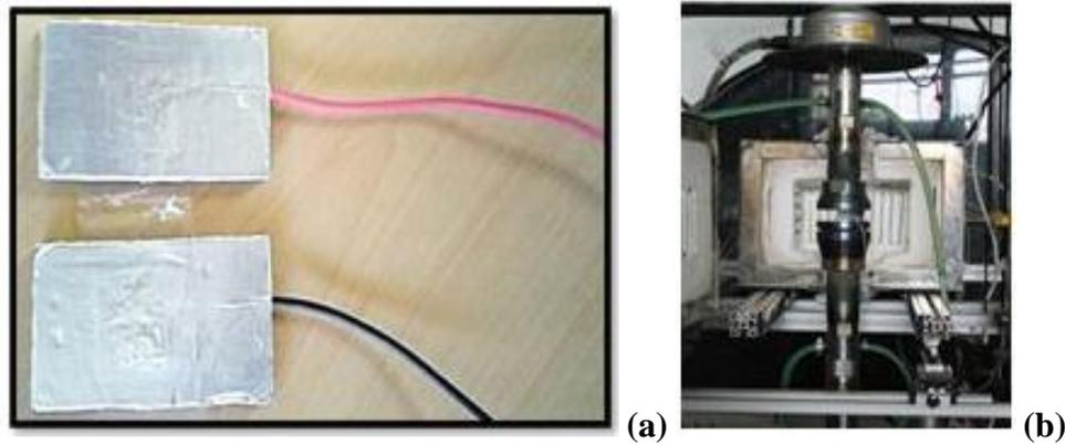
Figure 1): (a) Piezoelectric force sensing arrangements: aluminium electrodes for sandwiching the PVDF nanofibers; (b) ITW BISS UNO100 UTM machine for application of calibrated load.
