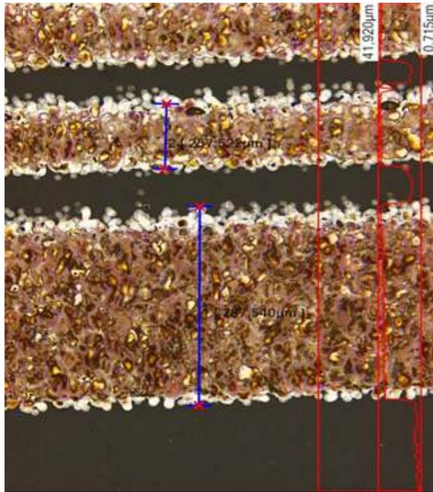
Figure (3): 3D-laser-scanning microscope-recording of the surface of inkjet printed resistive temperature sensor.
