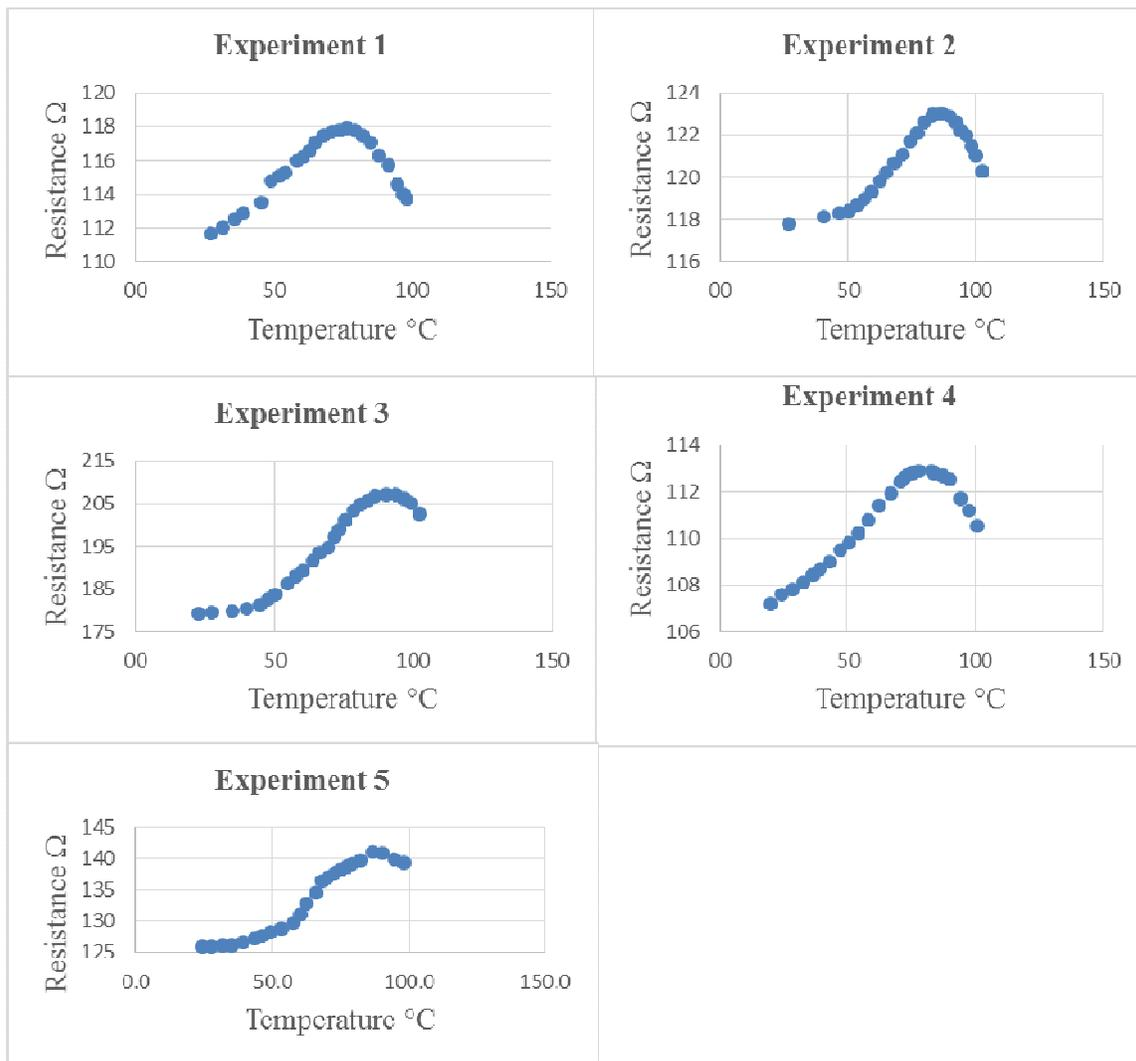
Figure (4): Functional relationship between resistance and temperature before temperature after treatment
