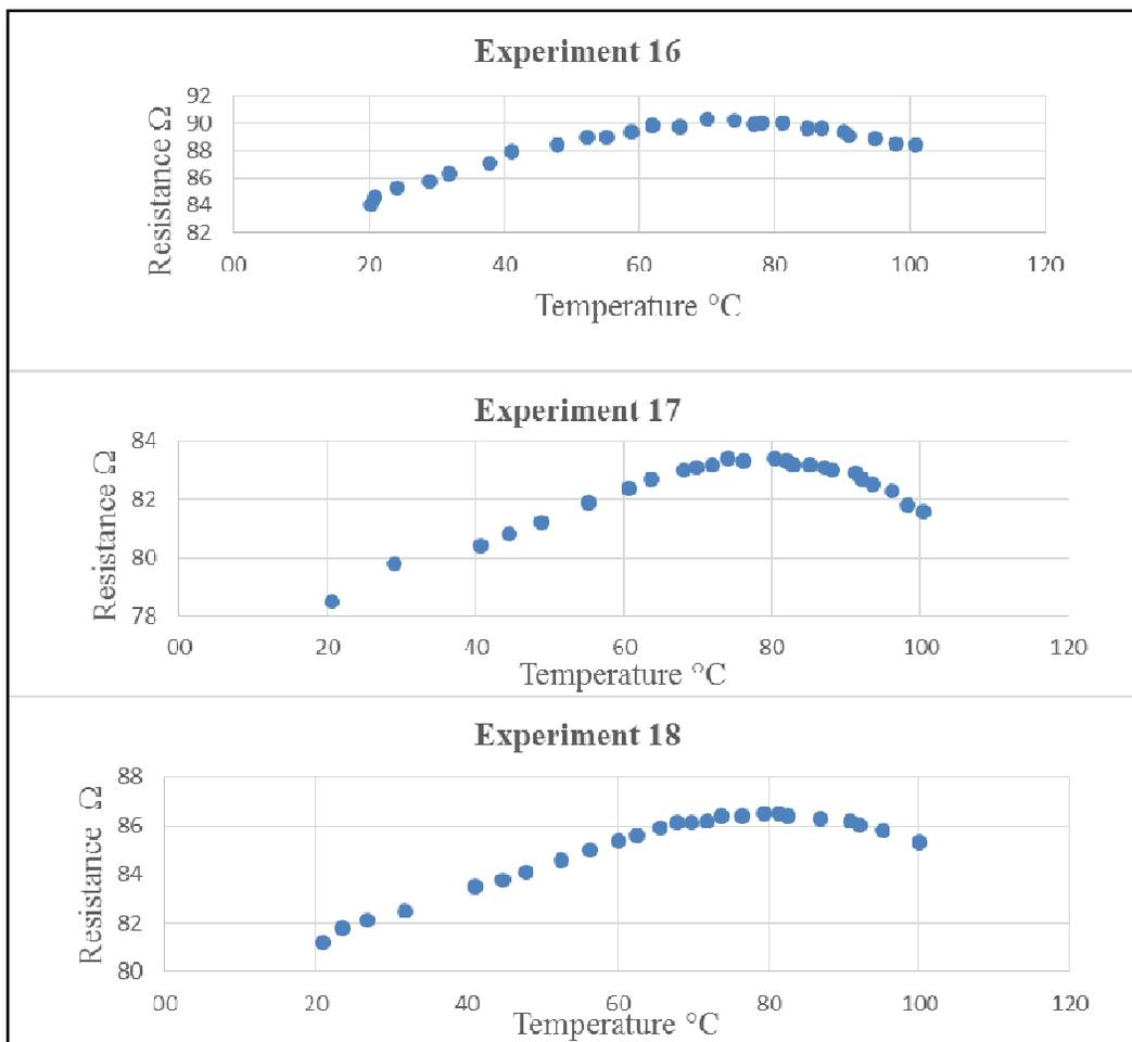
Figure (6): Functional relationship between resistance and temperature without temperature pre / post treatment with bending effect
