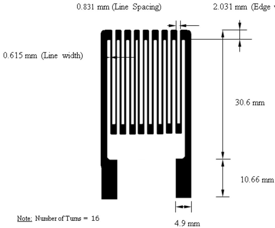
Figure (1): Design of the temperature sensor.
