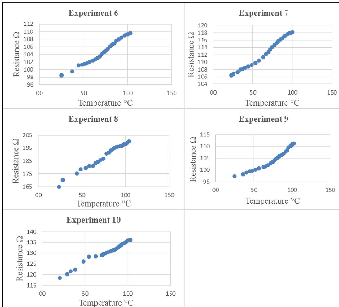
Figure (5): Functional relationship between resistance and temperature after temperature post- treatment.
