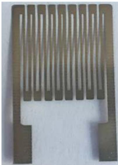
Figure (2): Fabricated inkjet printed resistive temperature sensor used for the experimental analysis.
