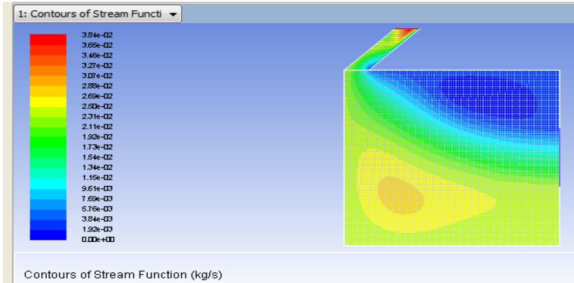
Figure (12a): Inlet at middle of the wall; Mass flow rate = 4.2158 kg/min.
