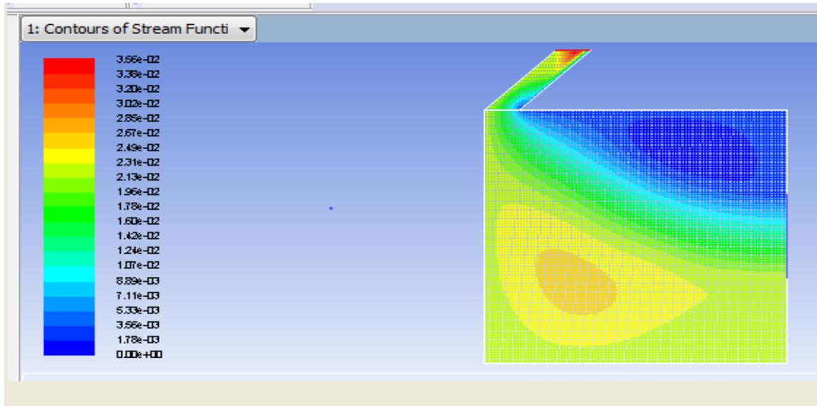
Figure (8): Contours of steam function for  $q=600 \text{ w/m}^2$ .
