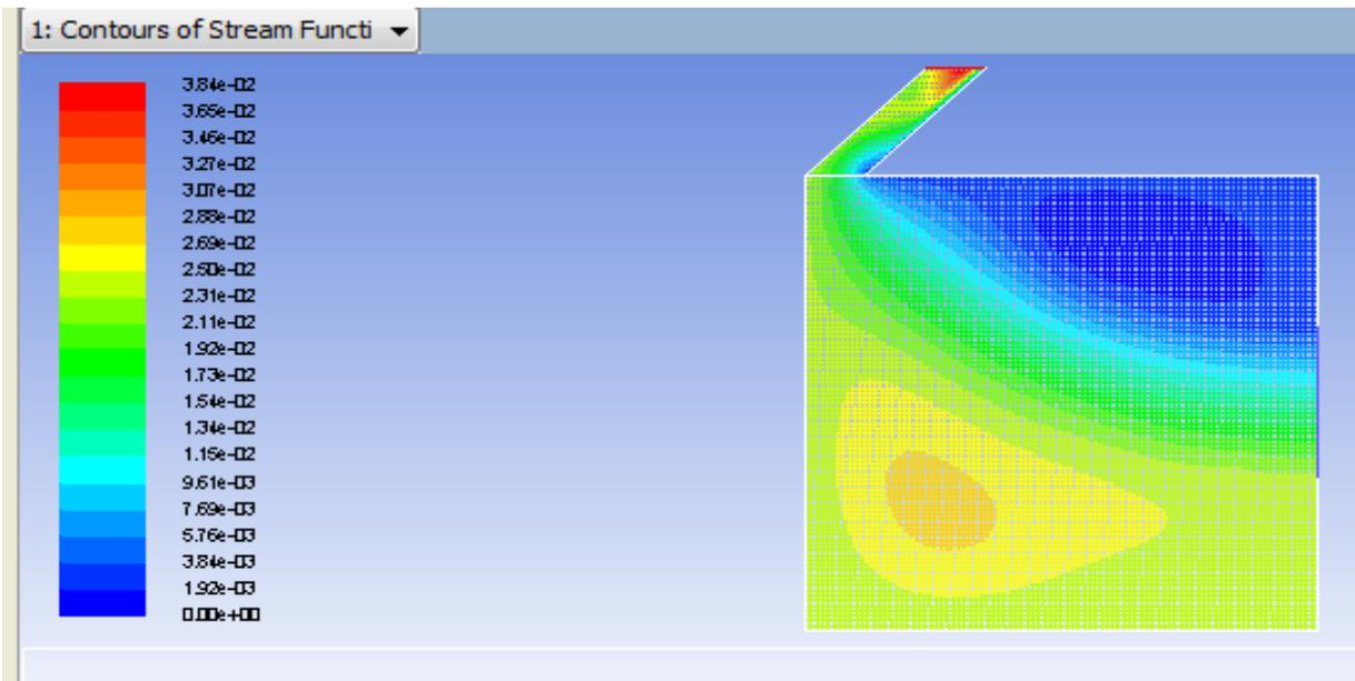
Figure (11): Contours of steam function for  $q=750 \text{ w/m}^2$ .
