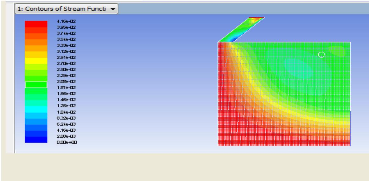
Figure (12c): Inlet at bottom of the wall; Mass flow rate=4.00 kg/min.
