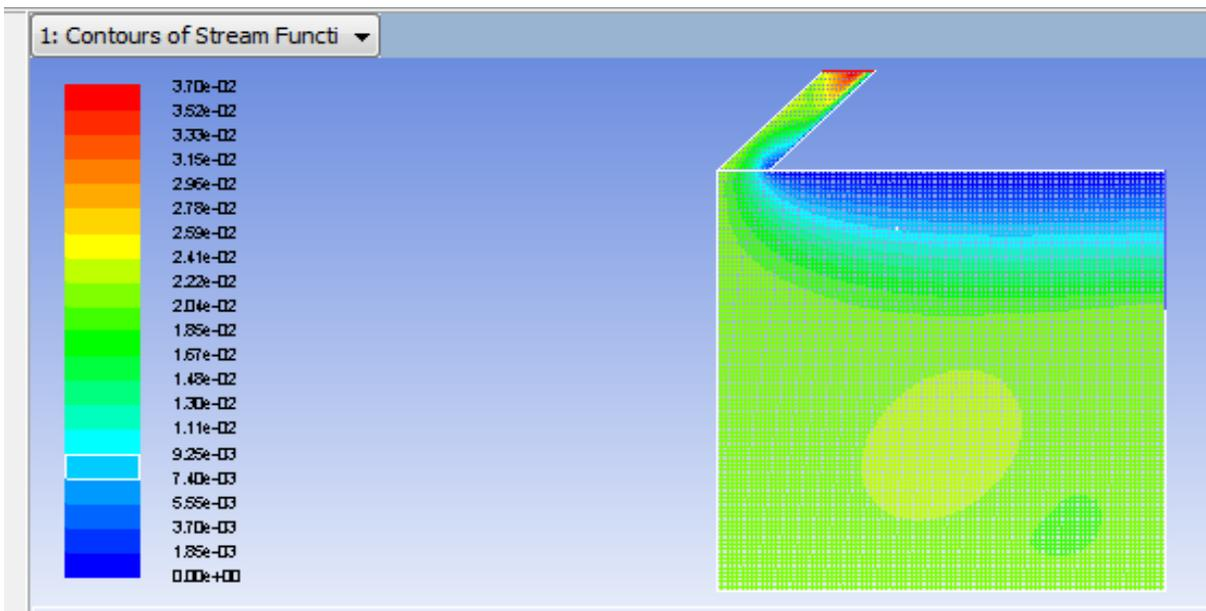
Figure (12b): Inlet at top of the wall; Mass flow rate=3.9641 kg/min.
