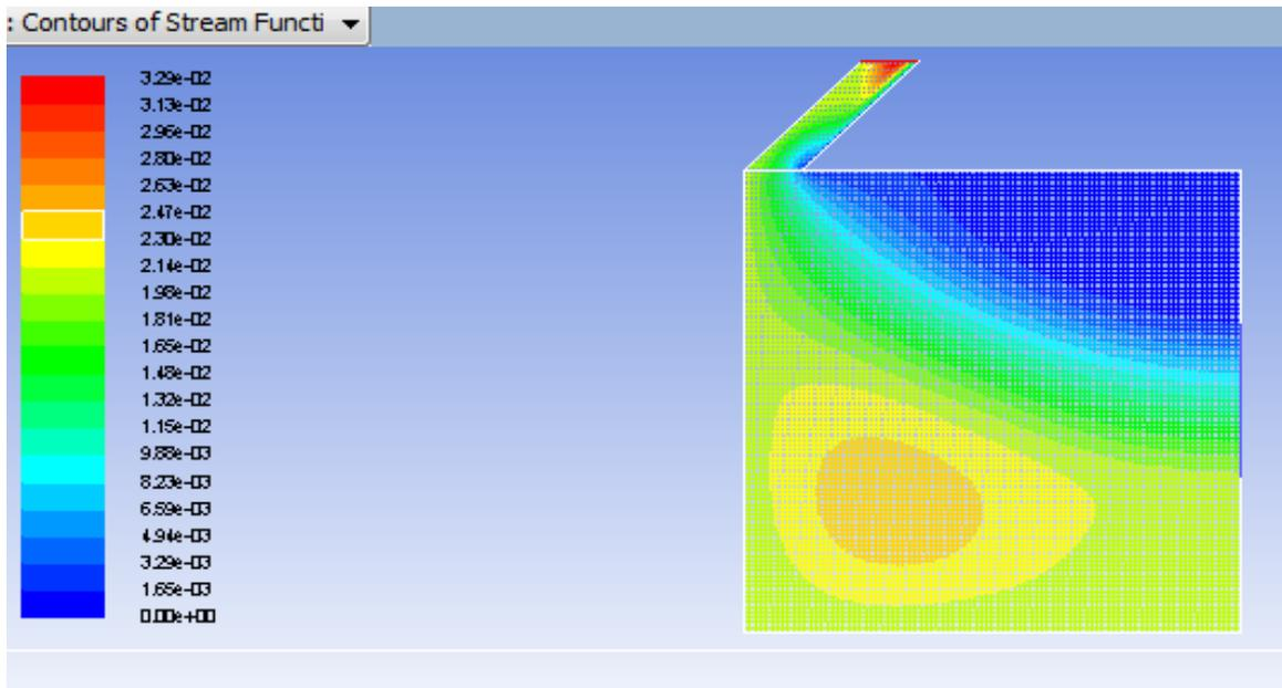
Figure (6): Contours of steam function for  $q=500 \text{ w/m}^2$ .
