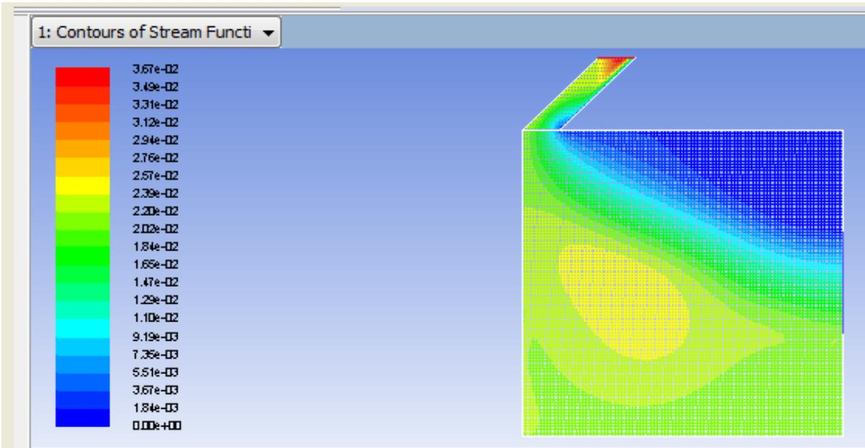
Figure (9): Contours of steam function for  $q=650 \text{ w/m}^2$ .
