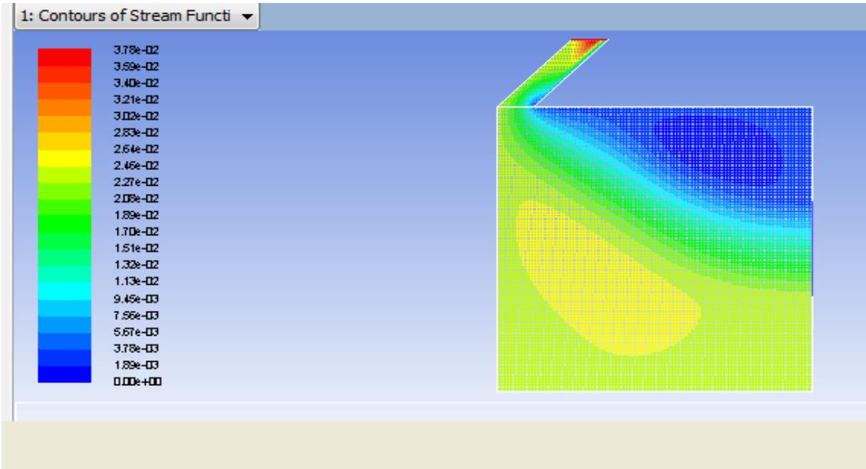
Figure (10): Contours of steam function for  $q=700 \text{ w/m}^2$ .
