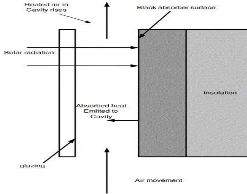
Figure (1): Schematic of solar chimney.
