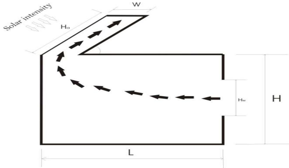
Figure (2): Room attached with inclined solar chimney.
