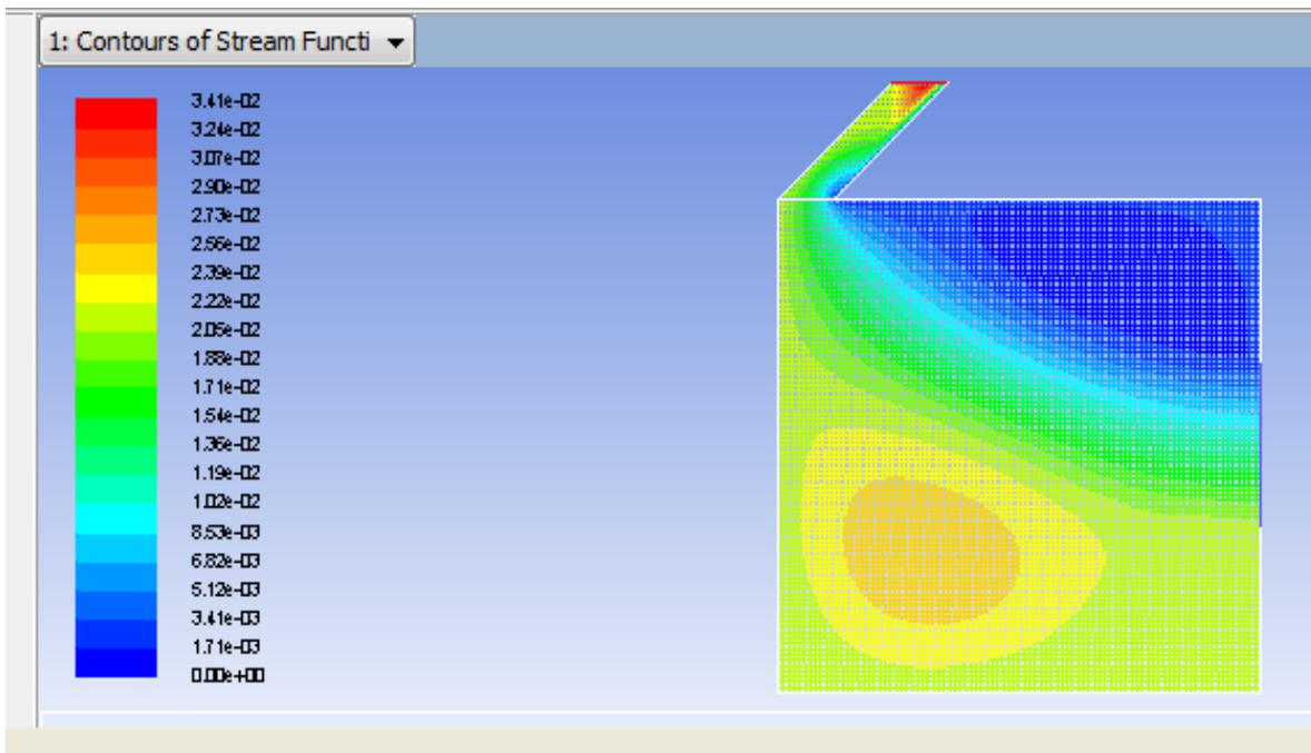
Figure (7): Contours of steam function for  $q=550 \text{ w/m}^2$ .
