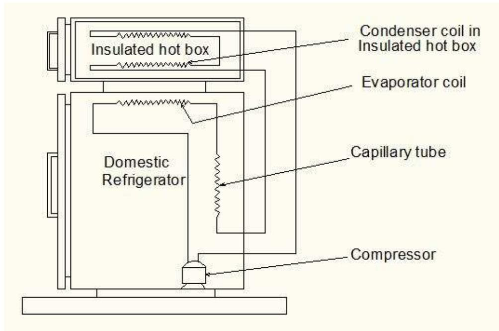
Figure (3): Schematic of waste heat utilization.
