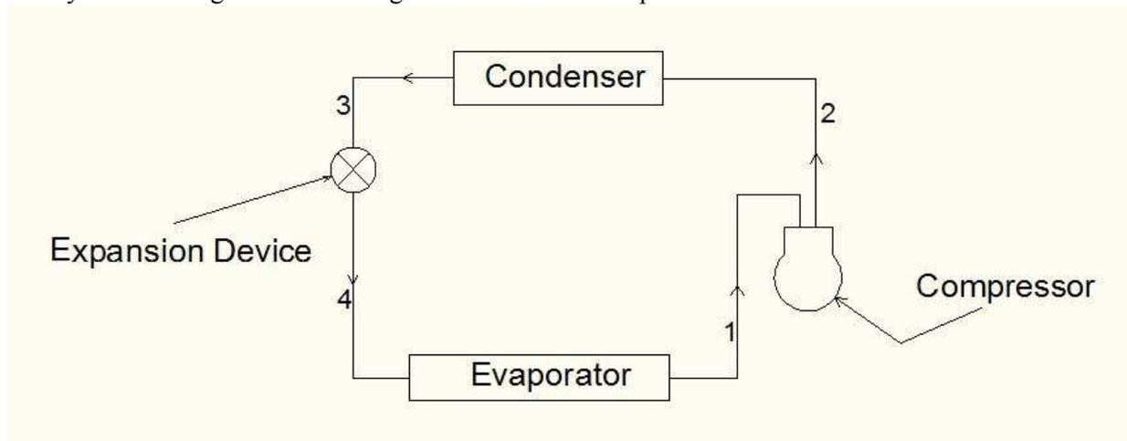
Figure (1): Flow diagram of refrigeration cycle.
