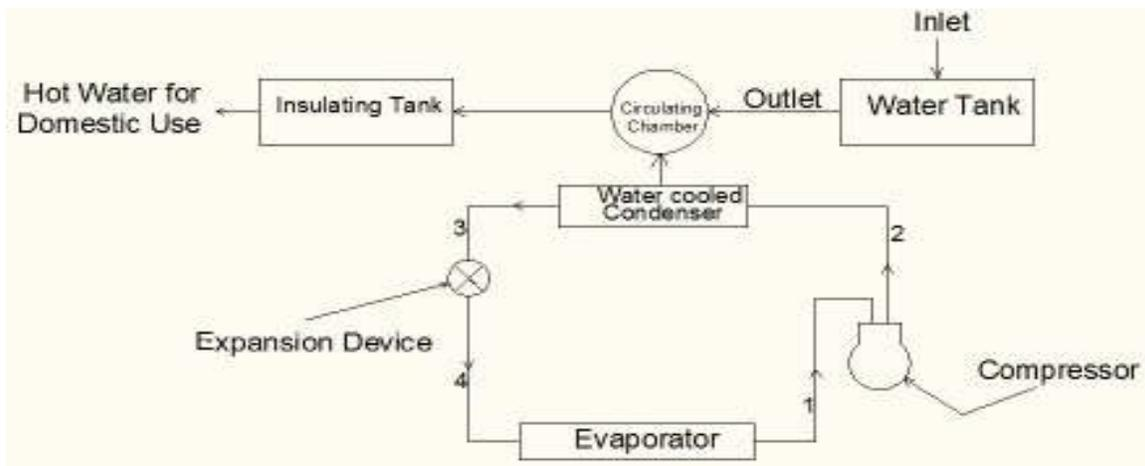
Figure (2): Waste heat utilized as water heating.
