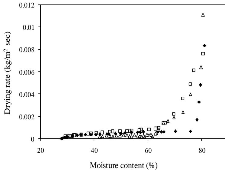
**Fig 3: Drying rate versus moisture content of POP at varied geometries. (□ square, △ cylinder, ◆ rectangle) Conditions : Initial moisture content 70%, Power -360 W**
