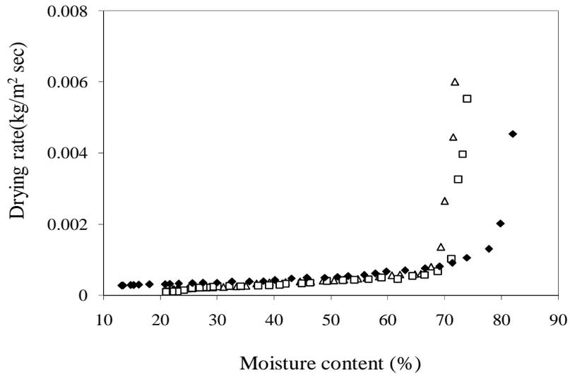
**Fig 2: Drying rate versus moisture content of POP at different initial moisture contents (□ Initial moisture content 75%, △ Initial moisture content 70%, ◆ Initial moisture content 80%) Conditions: Rectangle, Power 180W.**
