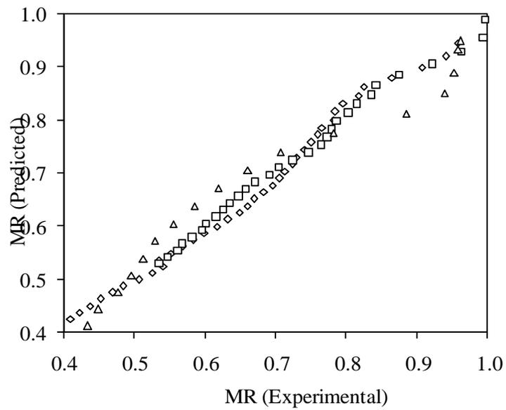
**Figure (5) : Predicted and experimental moisture content of POP during microwave drying (◇ Power 180W, □ Power 360 W, △ Power 540 W).**
