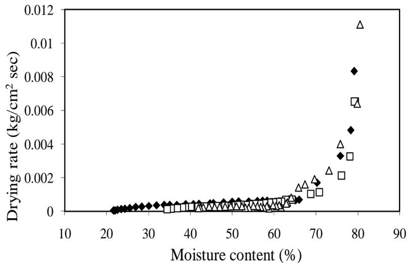
**Figure (1) : Drying rate versus moisture content of POP at different power ranges (♦,P-180W, □,P- 360W, △,P-540W) Conditions: Initial moisture content-70%, Geometry- Cylinder**
