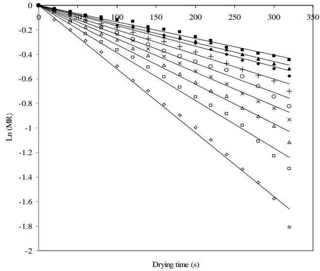
**Figure (6) : Drying kinetic relationship of POP at different microwave power ranges for 13 mm sample thickness:  $\diamond$  - 180 W, IM 80%;  $\square$ , 360 W, IM 80%;  $\triangle$ , 180 W, IM 75%;  $\times$ , 180 W, IM 70%;  $\circ$ , 360 W, IM 75%;  $+$ , 540 W, IM 75%;  $\blacklozenge$ , 540 W, IM 80%;  $\blacktriangle$ , 360 W, IM 70%;  $\blacksquare$ , 540 W, IM 70%.**
