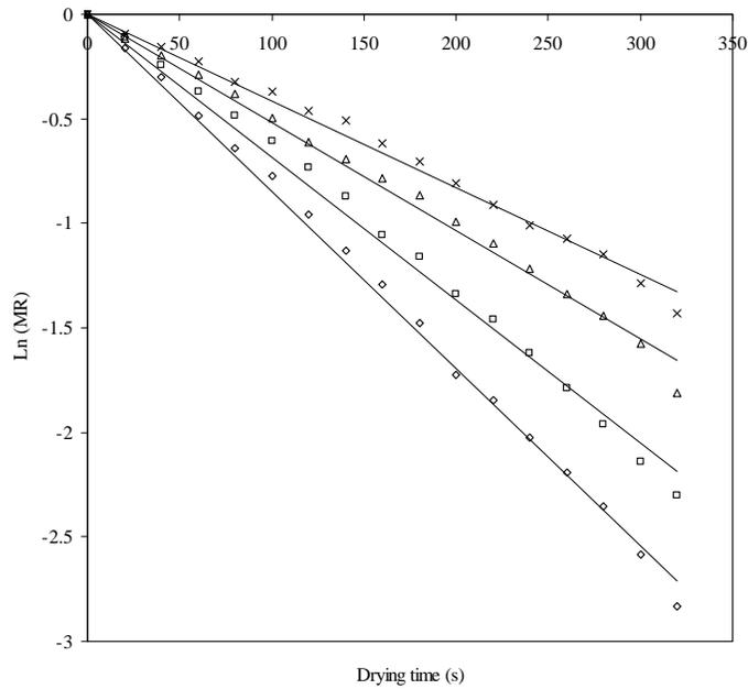
**Figure (7) : Drying kinetic relationship of POP at different sample thickness for microwave power 180 W and IM 80.  $\diamond$ , 14 mm;  $\square$ , 13mm;  $\triangle$ , 12mm;  $\times$ , 11mm.**
