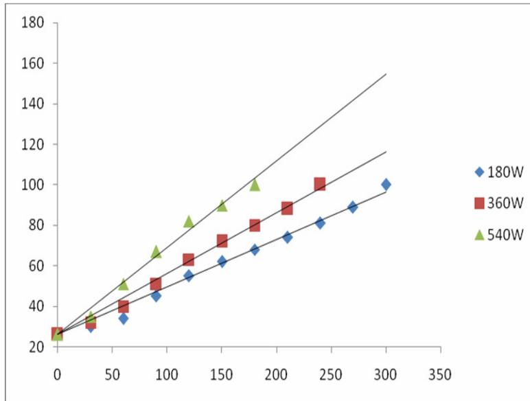
Figure (3) : Temp (C) Vs Time (S). Effect of power dependent microwave heating of water : ♦ 180W: ■ 360W: ▲ 540W
