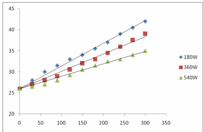
Figure (2) : Temp (C) Vs Time (S). Effect of power dependent microwave heating of plaster : ◆ 180W: ■ 360W: ▲ 540W
