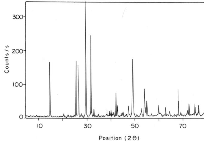
Figure (5a) : XRD pattern of plaster before Microwave irradiation.
