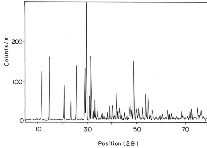
Figure (5b) : XRD pattern of plaster after Microwave irradiation.
