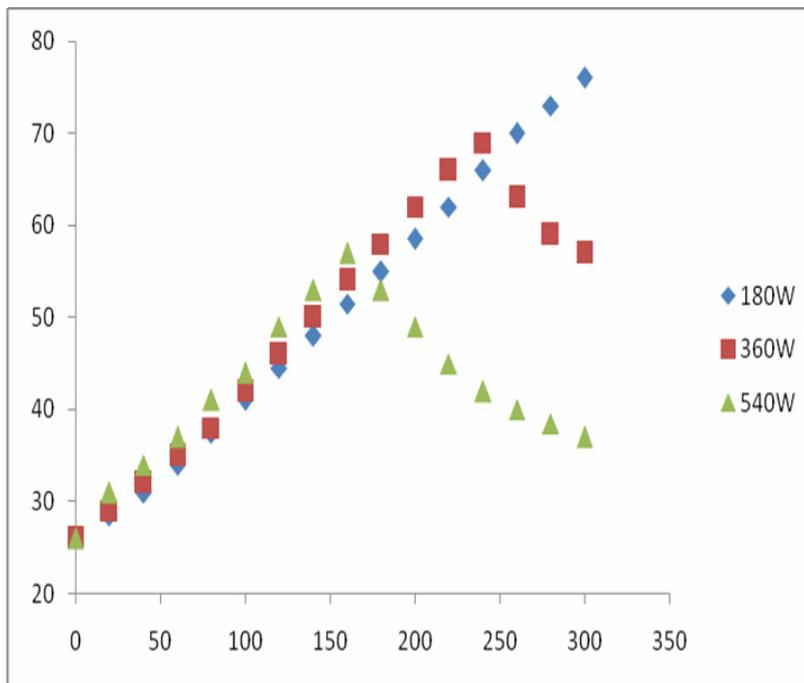
Figure (4) : Temp(C) Vs Time (S). Effect of power dependent microwave heating of water on plaster : ♦ 180W: ■ 360W: ▲ 540W
