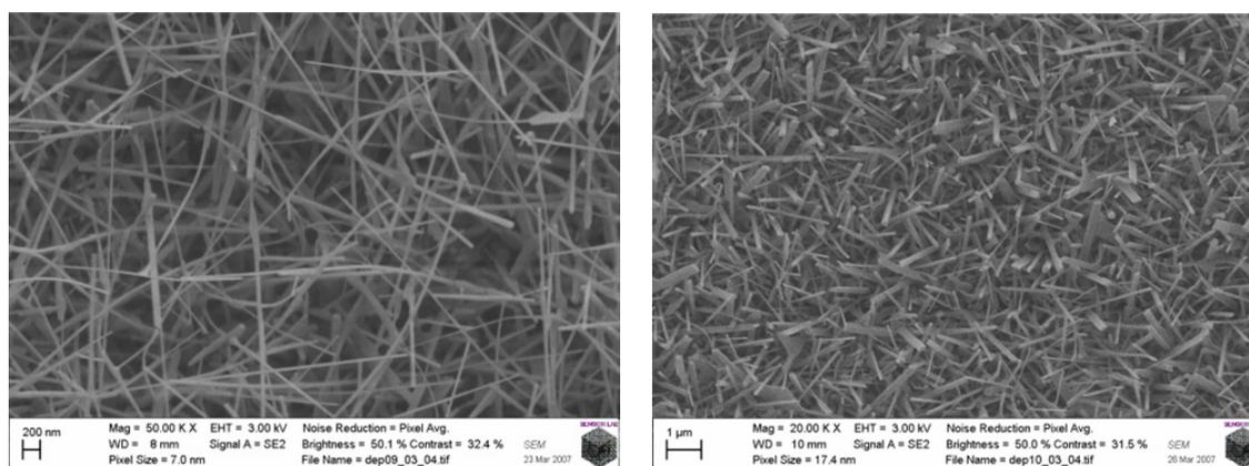
Figure (2) : Zinc oxide nanowires deposited with Pt (left) and Pd (right) catalyst at a deposition temperature of 320-340°C.
