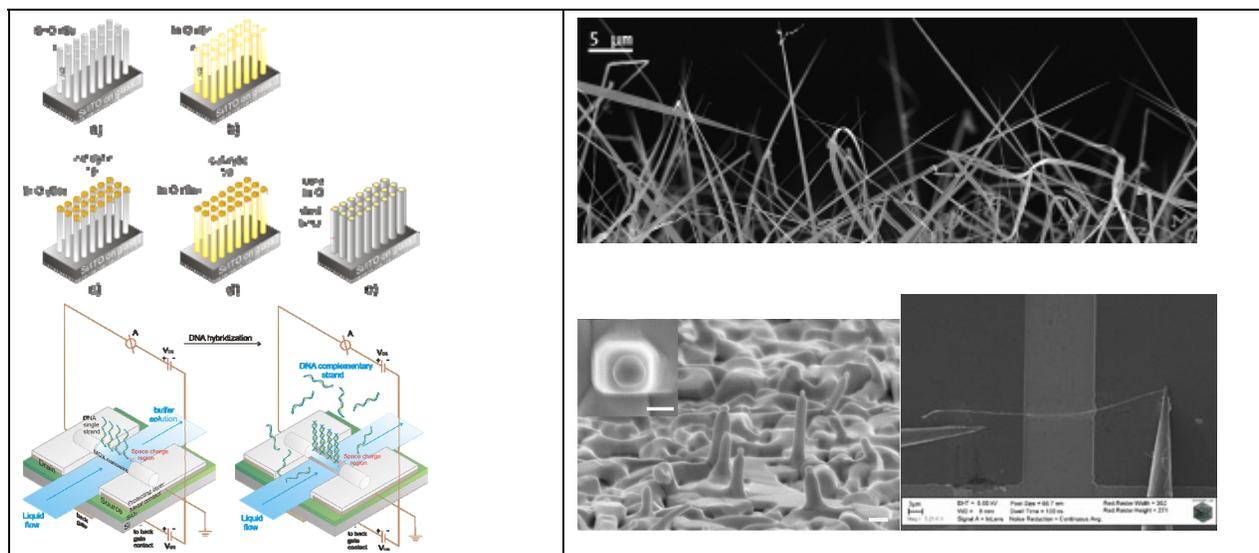
Figure (1) : Left up: Nanowire based structures aligned arrays of a) b), same structures via a growth catalyst c) and d), core-shell structure e). Left down: Single Nanowire Transistor for biosensing. Right up: SEM image of a bundle of nanowires. Right down: SEM image of  $\text{In}_2\text{O}_3$  nanowires grown on sapphire incorporating the catalytic seed cluster (here Au) on top and of a single nanowire placed between two contacts by nanomanipulation.
