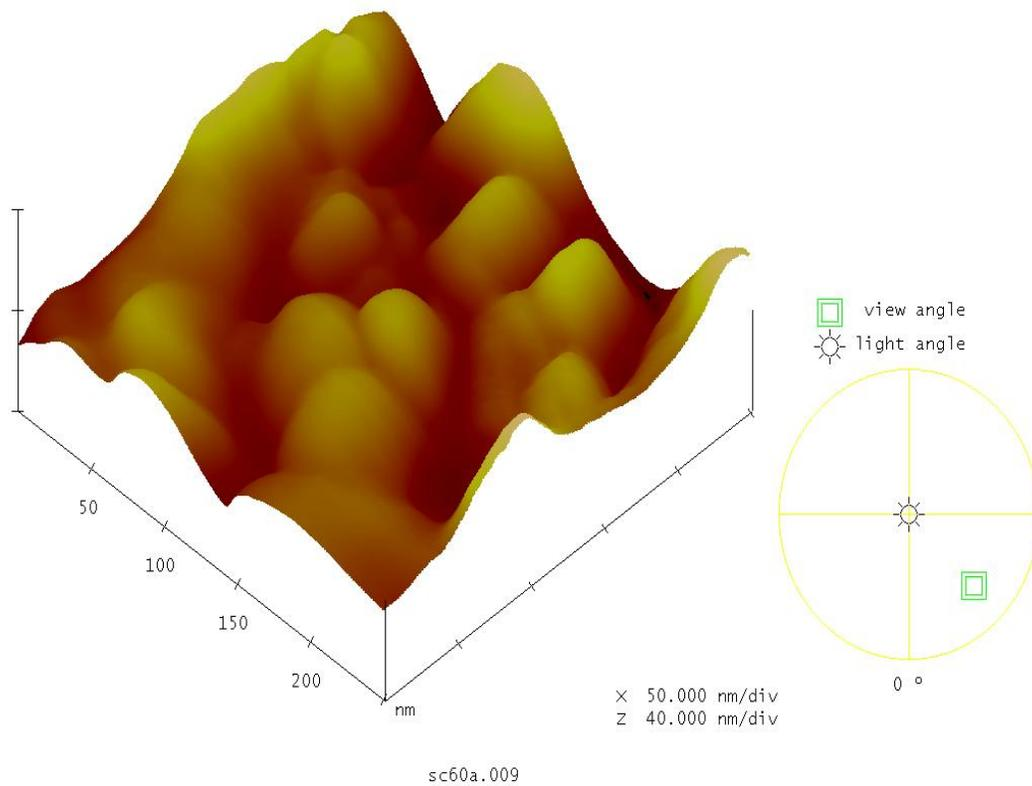
Figure 2 : AFM image of YBCO/LLDPE composite sample.
