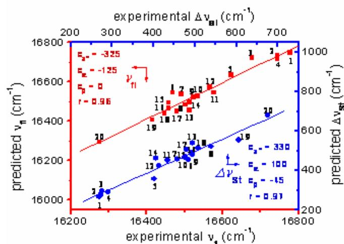
Figure (11) : Multiple linear regression of the fluorescence wavenumber and Stokes shift of PM650 in a wide variety of solvents using the Taft solvent scales (from apolar 1 to polar/protic 20, see Table 3) [138].
