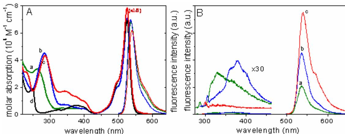
Figure (8) : (A) Absorption and fluorescence (under Vis excitation) spectra of P2ArAc (a), P3ArAc (b) and P3ArP (c) in *c*-hexane. The corresponding spectrum of PM567 (d) is also included for comparison. (B) Fluorescence spectra under UV excitation [119, 120].
