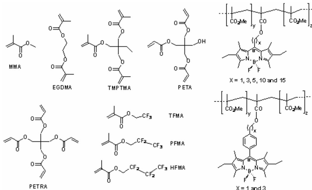
Scheme (2) : Molecular structure of the monomers and dye linkage to the PMMA chain through a linear spacer of different length or by a *para* substituted phenyl groups [99,100, 102, 104].
