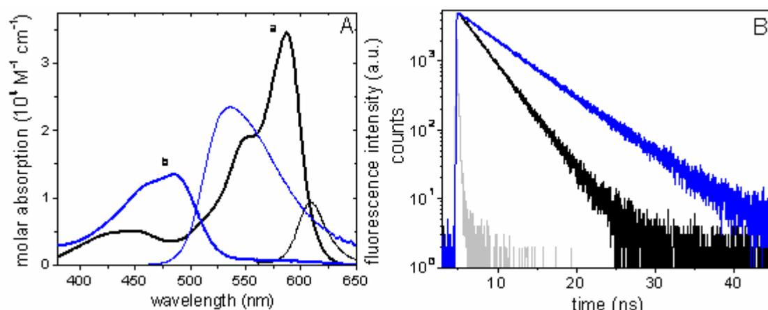
Figure (13) : A) Absorption and fluorescence (scales by their  $\phi$  value) and B) fluorescence decay curves of PM650 in acetone (a) and DMF (b) [140].
