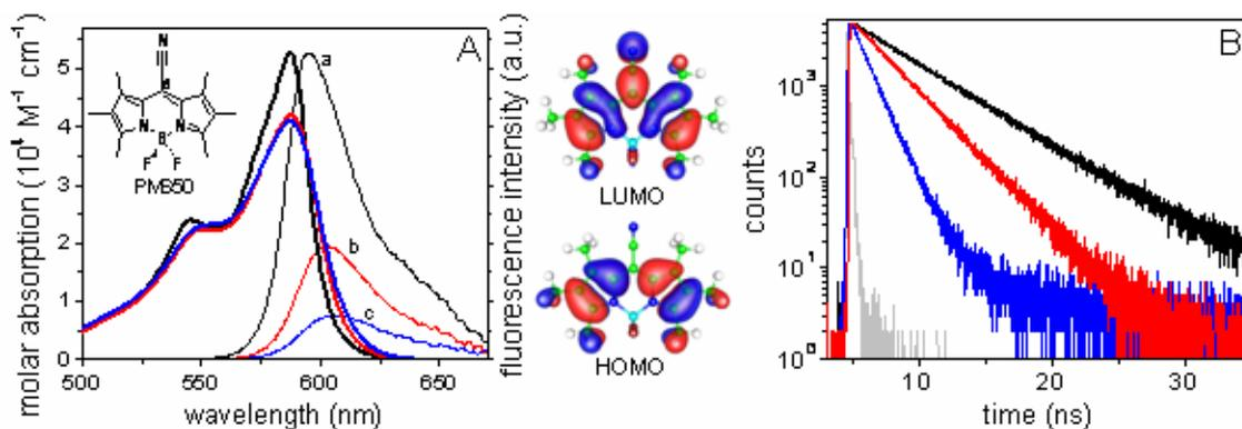
Figure (10) : (A) Absorption and fluorescence of PM650 in diluted solutions of c-hexane (a), dioxane (b) and methanol (c). (B) Fluorescence decay curves of the dye in those solvents.
