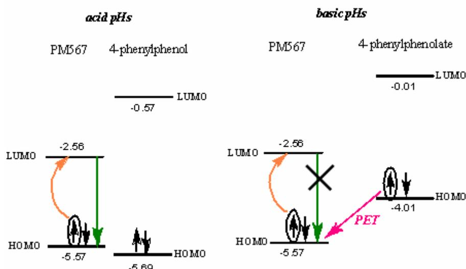
Scheme (6) : Calculated energy (in eV) of the frontier orbitals of PM567 and 4-phenylphenol in its neutral (acid pHs) and ionized (basic) forms in ethanol [120].
