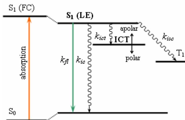
Scheme (5) : Energy diagram for the deactivation processes from the  $S_1$  excited state of PM650: LE (Localized Excited), FC (Franck–Condon) and ICT (Intramolecular Charge Transfer) states. Continuous and dotted lines represent radiative and non-radiative processes, respectively [138].
