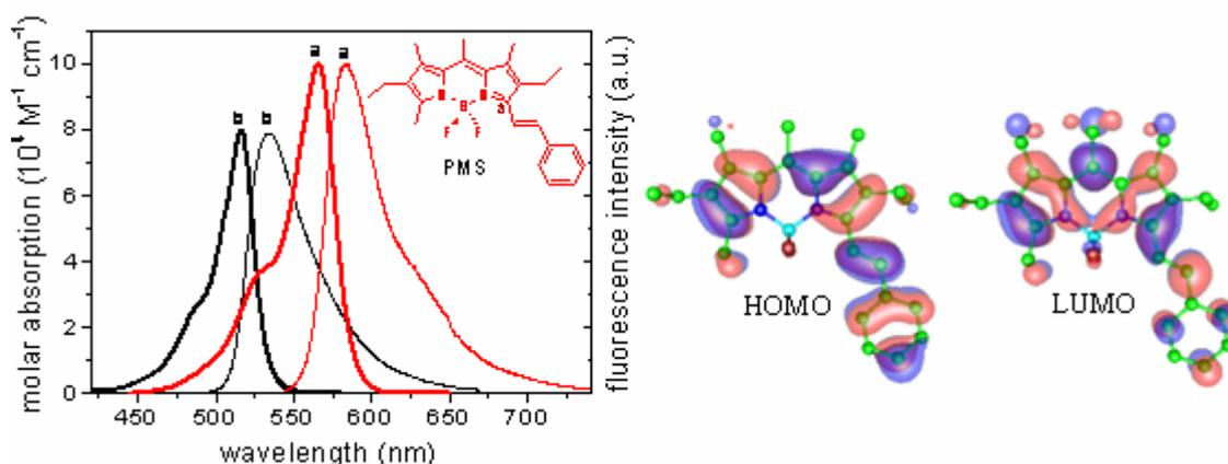
Figure (6) : Normalized absorption and fluorescence spectra of PMS (a) and PM567 (b) in diluted solutions of methanol [115]. The contour maps of the HOMO and LUMO of PMS are also included.
