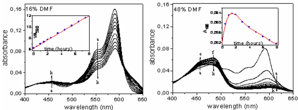
Figure (14) :Evolution of the absorption spectra with the ageing time, from 0 (a) to 8 hours (k), of PM650 in DMF/dioxane mixtures (left 16 % and right 48 % in DMF) [140]. Inset shows evolution of the absorbance at specific absorption wavelengths with the ageing time.
