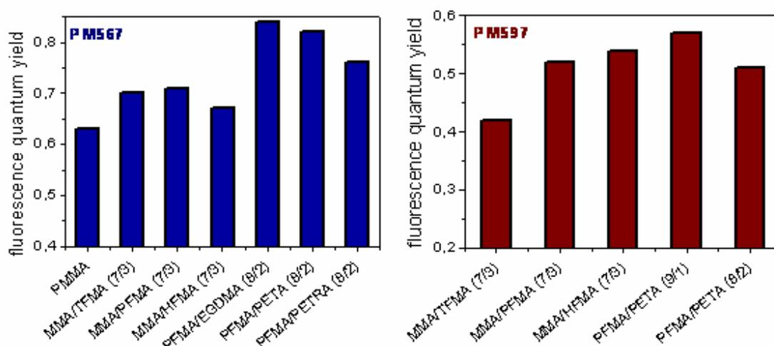
Figure (5) : Evolution of the fluorescence quantum yield of PM567 and PM597 with the type and proportion of fluorinated and crosslinked copolymers [103] (*nomenclature in Scheme 2*).
