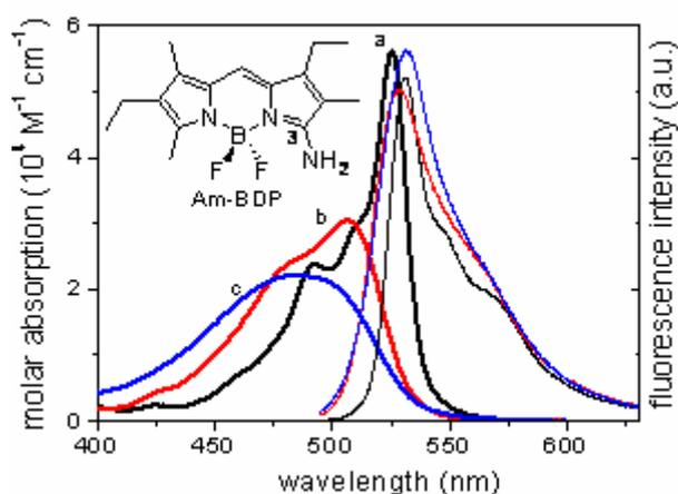
Figure (15) : Absorption and fluorescence spectra of 3–amino BODIPY (Am–BDP) in diluted solutions of *c*–hexane (a), ethyl acetate (b) and trifluoroethanol (c) [116, 117].
