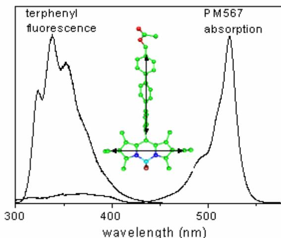
Figure (9) : Spectral overlap of the normalized absorption spectrum of PM567 and fluorescence band of terphenyl group. Inset: mutual orientation of the transition moments of each dye in P3ArAc [120].
