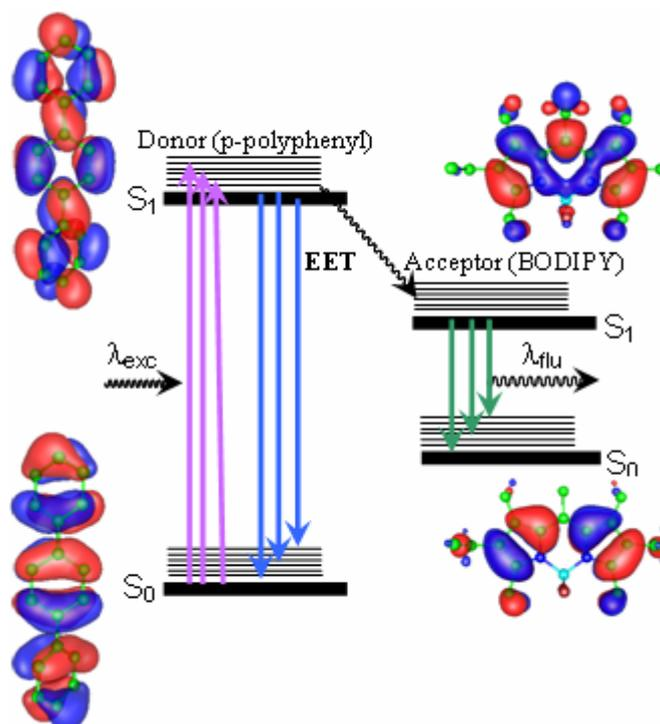
Scheme (4) : Intra-EET mechanisms in PXArAc and P3ArP dyes, together with the electronic density in the HOMO and LUMO states of PM567 and *p*terphenyl dyes [120].
