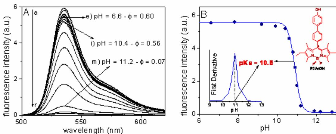
Figure (18) : Fluorescence spectra evolution of P2ArOH with the solvent basicity in ethanol [120] (from pH = 0 (a) to pH = 13.1 (r)).
