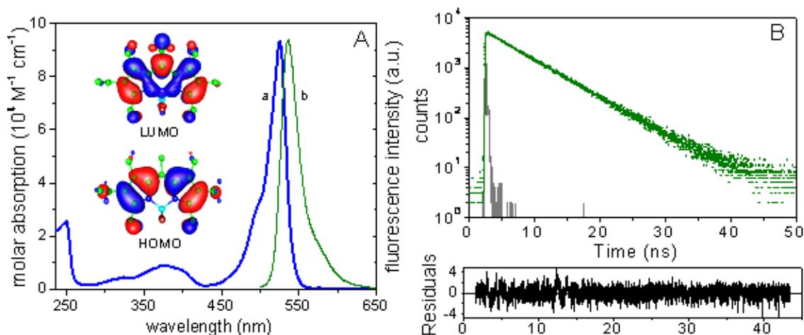
Figure (1) : (A) Absorption (a) and fluorescence (b) spectra and (B) fluorescence decay curve (top) and residuals.(bottom) of PM567 in diluted solutions ( $2 \times 10^{-6} \text{ M}$ ) of c–hexane [78].
