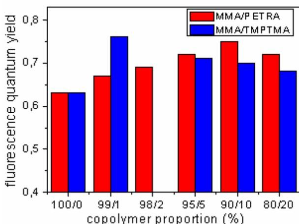
Figure (4) : Evolution of the fluorescence quantum yield of PM567 with the concentration of the crosslinking agent (PETRA and TMPTMA) in the copolymer with MMA [101].
