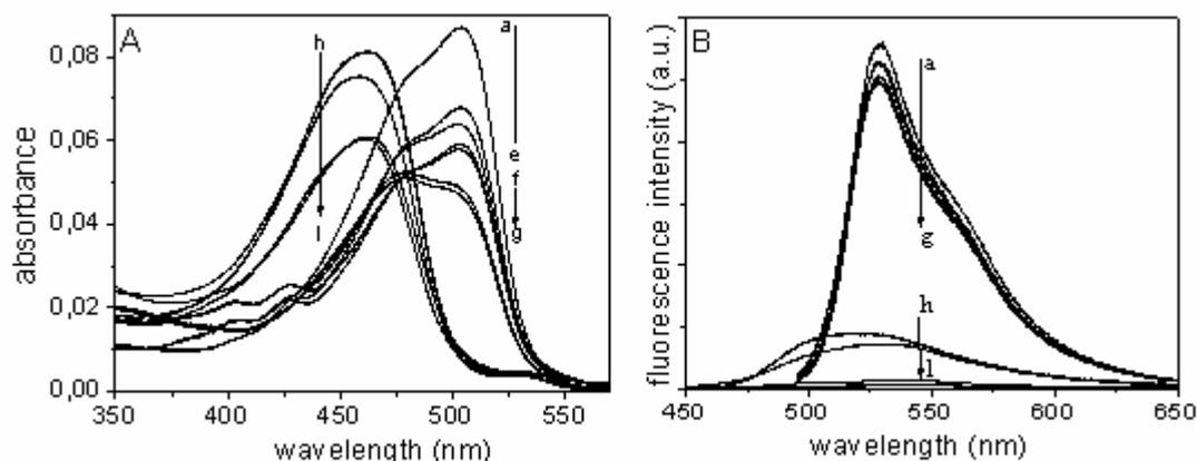
Figure (16) : Absorption (A) and fluorescence (B) spectra of 3-amino BODIPY in acid and basic ethanolic solutions [117] (from  $[\text{OH}^-] = 3 \times 10^{-3}$  M (a) to  $[\text{H}^+] = 3 \times 10^{-6}$  M (e), from  $[\text{H}^+] = 4 \times 10^{-5}$  M (f) to  $[\text{H}^+] = 4 \times 10^{-4}$  M (g) and from  $[\text{H}^+] = 2 \times 10^{-3}$  M (h) to  $[\text{H}^+] = 8 \times 10^{-2}$  M (l)).
